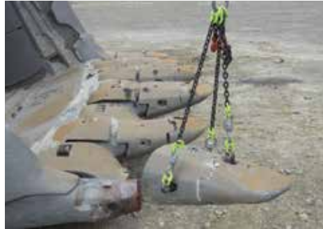
ESCO SecureLift™ system for safer removal.
